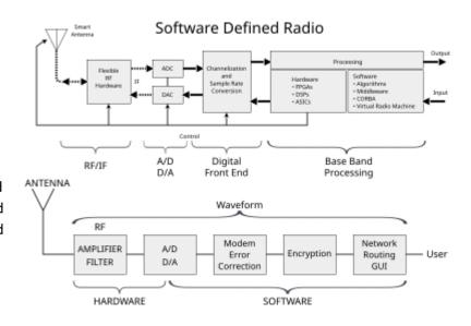
ADC or A/D = Analog to Digital Converter; DAC or D/A = Digital to Analog Converter
